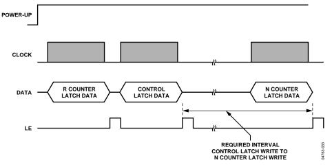
Figure 21. ADF4360-8 Power-Up Timing
