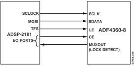
Figure 26. ADSP-2181 to ADF4360-8 Interface
