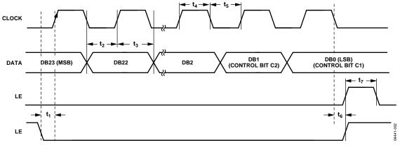
Figure 2. Timing Diagram
