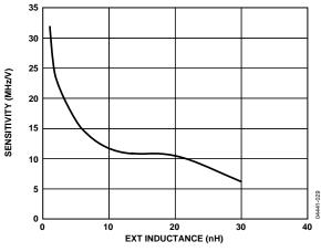
Figure 25. Tuning Sensitivity (in MHz/V) vs. Inductance (nH)
