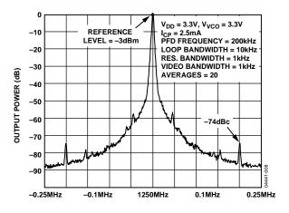
Figure 8. Reference Spurs at 500 MHz (200 kHz Channel Spacing, 10 kHz Loop Bandwidth)
