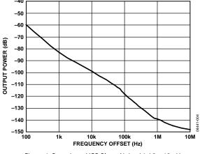
Figure 4. Open-Loop VCO Phase Noise, L1, L2 = 13 nH
