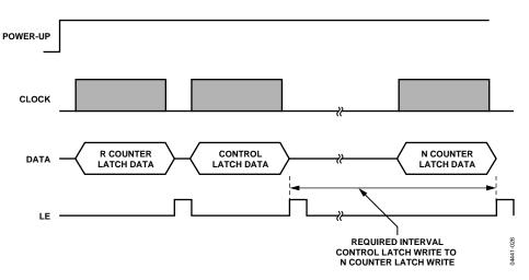
Figure 22. ADF4360-7 Power-Up Timing
