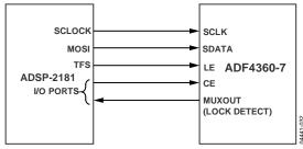
Figure 28. ADSP-2181 to ADF4360-7 Interface
