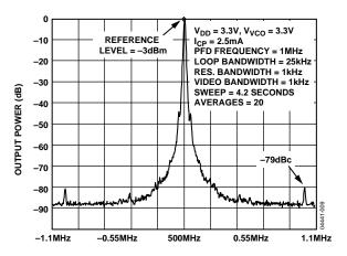
Figure 9. Reference Spurs at 500 MHz (1 MHz Channel Spacing, 25 kHz Loop Bandwidth)
