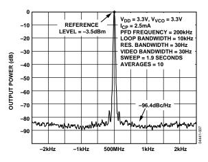
Figure 7. Close-In Phase Noise at 500 MHz (200 kHz Channel Spacing)
