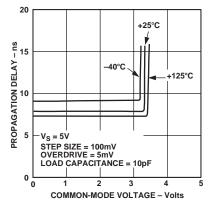
Figure 8. Propagation Delay vs.  $V_{CM}$
