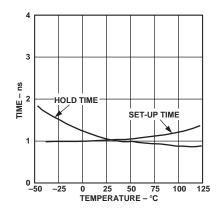
Figure 9. Latch Setup-and-Hold Time vs. Temperature
