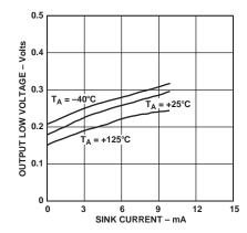
Figure 10. Output Low Voltage, V<sub>OL</sub> vs. Sink Current
