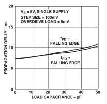
Figure 4. Propagation Delay vs. Load Capacitance
