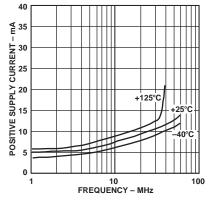
Figure 14. Positive Supply Current vs. Frequency
