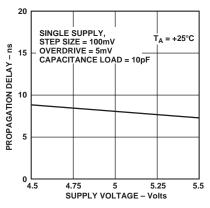
Figure 6. Propagation Delay vs. Positive Supply Voltage
