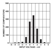
*Figure 2. Typical Distribution of Input Offset Voltage*
