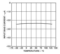
*Figure 16. Input Bias Current vs. Temperature*
