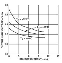
Figure 11. Output High Voltage,  $V_{OH}$  vs. Source Current
