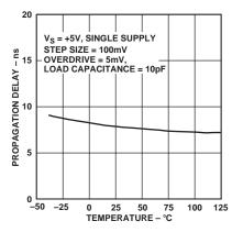
Figure 7. Propagation Delay vs. Temperature
