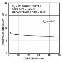
*Figure 3. Propagation Delay vs. Overdrive*
