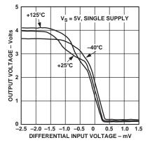
Figure 1. Output Voltage vs. Differential Input Voltage
