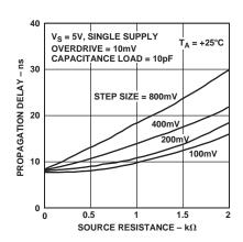
*Figure 5. Propagation Delay vs. Source Resistance*
