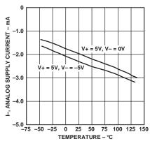
Figure 12. Analog Supply Current vs. Temperature for +5 V, –5 V Supplies
